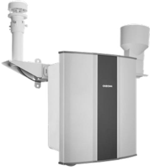
Weathercom® measures meteorological parameters such as wind speed and direction, rainfall, visibility, UV-radiation, light intensity, temperature, humidity, pressure, etc. Through Weathercom®, hyper-local meteorological parameters can be monitored in real-time which can help to take on-time decisions in case of any natural hazard. Weather forecasting and predictions is possible through historical data and trend analysis which can aid in timely warning / alert broadcasting.
